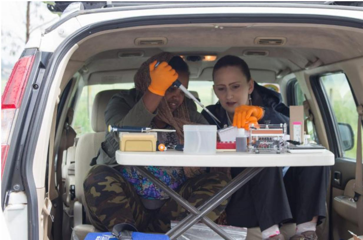
The mobile lab allows researchers to extract and prepare rust DNA for sequencing in the field. Photo provided by John Innes Centre.
